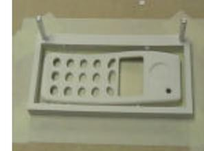
Using a hobby knife, the model is removed from the frame.
