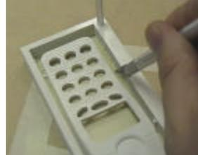
Coating agent is added to harden the model. Allow to dry and finish.
